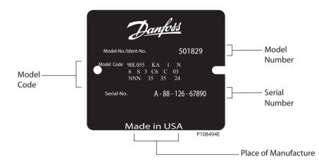
Series 90 pumps are also manufactured in Europe and China. Place of manufacture shown on nameplate will correspond with the actual place of manufacture.
